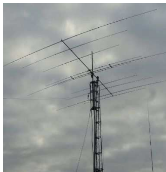
De nieuwe beam: full size 3 ele 20m & 15m / 4 ele op 10m Zonder traps - Sleeve fed design - SWR 'plat' !
